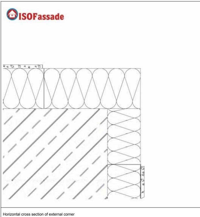
The corner piece is made on site and is to be covered with the rendering system
