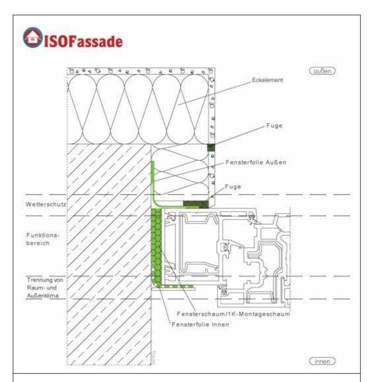
The application of a corner element and the use of an infill element between window and corner element Joint between infill element and corner element is sealed with silicon sealant
